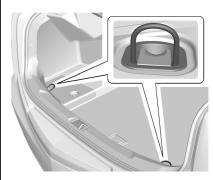
The cargo tie-downs can be used to secure small loads inside the trunk.
