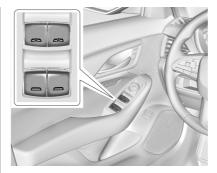
Power windows work when the ignition is on, in ACC/ACCESSORY, or when Retained Accessory Power (RAP) is active. See *Retained Accessory Power (RAP)* ⇒ 165.
