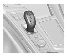
The shift pattern is displayed in the top of the shift lever. The selected gear position will illuminate red on the shift lever, while all others will be displayed in white. If the shift is not immediate, as in very cold conditions, the indicator on the shift lever may flash until it is fully engaged.
