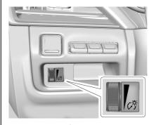
The brightness of the instrument panel lighting and steering wheel controls can be adjusted.
