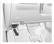
1. Pull the hood release lever with the symbol. It is on the lower left side of the instrument panel.
