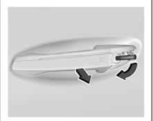
3. Insert the mechanical key in the cylinder.
