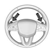
Vehicles with Tap Shift have controls on the back of the steering wheel to manually shift the automatic transmission.
