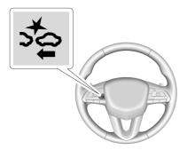
The Collision Alert control is on the steering wheel. Press to set the FCA timing to Far, Medium, or Near,
