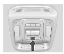
It is recommended that the intrusion and inclination sensor be deactivated if pets are left in the vehicle or the vehicle is being transported. With the vehicle turned off, press in the front overhead console. The indicator light will come on momentarily,
