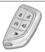
**1**: Press to lock all doors and the fuel door, if equipped. The turn signal indicators may flash and/or the horn may sound on the second press to indicate locking. See *Vehicle*Personalization ⇒ 121
