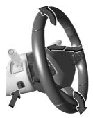
If equipped, the control is on the left side of the steering column.
