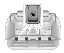
The lower anchors are located under the labeled covers on the seat cushion near the crease between the seatback and the seat cushion.
