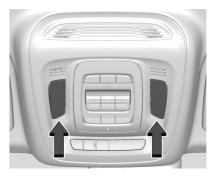
Press the lamp lenses on the front reading lamps.
