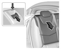
Pull the lever on top of the seatback toward you to unlock the seatback
