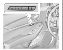
If equipped, memory seats allow two drivers to save and recall their unique seat positions for driving the vehicle, and a shared exit position for getting out of the vehicle. Other feature positions may also be saved, such as power mirrors and power steering wheel, if equipped. Memory positions are linked to remote key 1 or 2 for automatic memory recalls.
