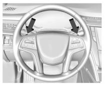
Tap Shift allows the driver to manually control the automatic transmission. To use Tap Shift, the shift lever must be in M (Manual Mode). If equipped, the controls are on the back of the steering wheel. Tap the left control to downshift, and the right control to upshift. A Driver Information Center (DIC) message indicates the gear the vehicle is in. See *Manual Mode* ⇔ 180.
