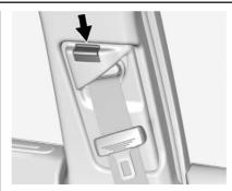
Push down on the release button and move the height adjuster to the desired position. The adjuster can be moved up by pushing the slide/ trim up.
