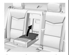
The rear seat has an armrest in the center of the seatback. Lower the armrest to access the cupholders.
