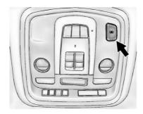
On vehicles with a rear window sunshade, the switch is on the overhead console. The sunshade only operates with the ignition on.
