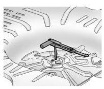
Turn the wrench counterclockwise to remove the fastener rod.
