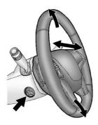
Press the control to move the tilt and telescoping steering wheel up and down or forward and rearward.
