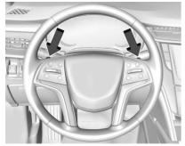
Tap Shift allows you to manually control the automatic transmission. To use Tap Shift, the shift lever must be in M (Manual Mode). The controls are on the back of the steering wheel.
