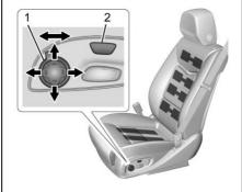
If equipped, the ignition must be on to use the massage feature.
