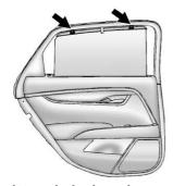
Attach it to the hooks at the top of the window.
