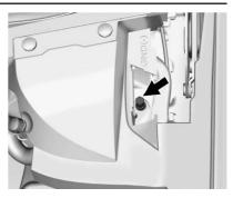
The vehicle has a remote negative (-) ground location. It is located on the driver side of the engine compartment. See *Engine Compartment Overview* ⇒ 224. Always use this remote ground location, instead of the terminal on the battery.
