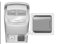
An indicator light on the outlet turns on to show it is in use. The light comes on when the ignition is on, equipment requiring less than 150 watts is plugged into the outlet, and no system fault is detected.
