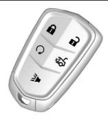
**a**: Press to lock all doors. The turn signal indicators may flash and/or the horn may sound on the second press to indicate locking. See *Vehicle Personalization* ⇒ 139.
