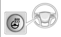
\*\* : If equipped with a heated steering wheel, press to turn on or off. An indicator next to the button is lit when the feature is turned on.
