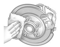
12. Remove any rust or dirt from the wheel bolts, mounting surfaces, and spare wheel.
