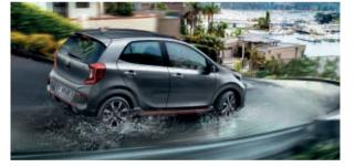
**Electronic Stability Control (ESC).** ESC ensures optimal braking performance and directional control. It automatically delivers the right amount of braking force to each wheel, based on an evaluation of engine torque and driving conditions.
