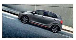
**Hill-start Assist Control.** When at a standstill on an incline, Hill-start Assist Control prevents you from rolling backwards. It applies the brakes from the time you lift your foot from the brake pedal, giving you a moment to switch your foot smoothly to the accelerator.
