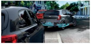
**Rear parking sensors.** Ideal for confident parking, these ultrasonic sensors mounted on the rear bumper warn you of any obstacles when manoeuvring into a parking space.
