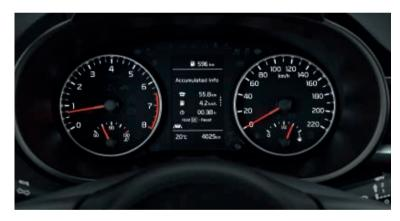
**4.2-inch supervision monochrome cluster display.** This screen is positioned between the rev counter and speedometer, and provides access to essential vehicle status, menus and trip data (grade dependent).
