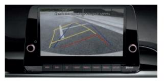
**Rear-view camera with dynamic guidelines.** The rear camera projects an image onto the 8-inch floating display, along with dynamic guidelines to help you into place.
