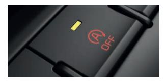
**Idle Stop & Go (ISG).** ISG comes as standard on all Picanto models and is designed to reduce fuel consumption by shutting down the engine when the vehicle is at a standstill.
