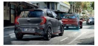
**Forward Collision-Avoidance Assist.** The system uses a frontfacing camera to guard against a collision with any vehicles or pedestrians ahead. By warning you and braking automatically, it can help you avoid, or reduce the severity of an accident.
