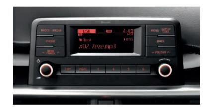
**Audio system.** The base audio system includes a 3.8-inch monochrome screen with DAB radio (grade dependent).
