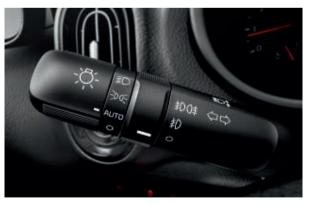
**Auto light control.** Set the stalk ring to Auto and the front and rear lights will turn on or off depending on lighting conditions.
