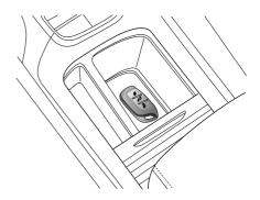
If the car is located in an area where there are strong radio signals causing interference or the smart key battery condition is low, please use the following steps to attempt to start the car:
