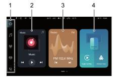
I Menu Bar: Displays 5 function icons. Click to enter the relevant function interface, and long press to customize the displayed items.
