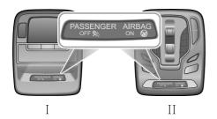
When the switch is turned to the ON position, the ON indicator light (located in the PAB display panel in the lamp assembly ) illuminates, this indicates that the passenger airbag is enabled.
