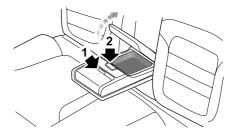
Fold forward to open the rear armrest. Press button I to open the cup holder. Press button 2 to open the storage box in the rear of the armrest.
