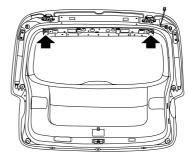
5 Pry off the screw trim cover, remove the 3 screws that fix the tailgate lower trim panel to the tailgate, pry off the snap, disconnect the harness connector, and remove the tailgate lower trim panel.
