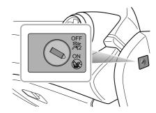
The passenger airbag switch is located in the right fascia panel end cover trim. Insert the key and rotate the switch to the on or off position to enable or disable the passenger airbag.
