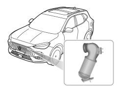
The exhaust system incorporates a catalytic converter, these help to convert poisonous exhaust emissions from the engine into environmentally less harmful gases. Catalytic converter is easily damaged through improper use, please observe the following precautions to minimise the chance of accidental damage.
