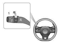
switch to return to position I. The indicator illuminates on the instrument panel when the rear fog lamps are on.
