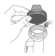
Check the washer fluid level regularly. When the level of washer fluid is low, please top up the washer fluid as instructed. Please use the washer fluid recommended and certified by the manufacturer. Refer to 'Recommended Fluids and Capacities' in "Technical Data" chapter.
