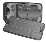
The vehicle features an emergency release device for the charging port lock.
