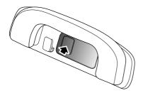
The rear courtesy lights are located on the left and right sides of interior roof panel. Press the lamp lens as indicated in the diagram to switch on the rear courtesy lights, press it again to switch off the lights.
