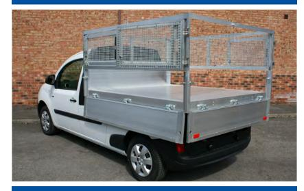
**ITEMS CAN BE PLACED IN TIPPER BODY BY OPENING SIDE OF CAGE**
