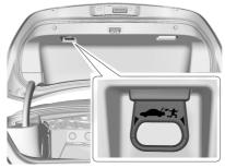
There is a glow-in-the-dark emergency trunk release handle on the trunk lid. This handle will glow following exposure to light. Pull the release handle to open the trunk from the inside.
