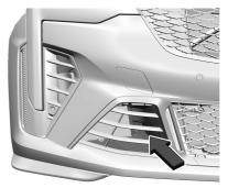
2. Front Brake Cooling Duct
