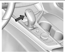
This vehicle is equipped with an electronic controlled transmission. The shift lock release button is designed to prevent inadvertent shifting out of P (Park) unless the ignition is on, the brake pedal is applied, and the shift lock release button is pressed.
