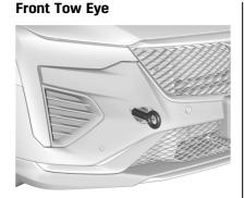
The vehicle is equipped with a tow eye. Only use the tow eye to pull the vehicle onto a flatbed car carrier from a flat road surface. Do not use the tow eye to pull the vehicle from snow, mud, or sand. The tow eye is located under the carpet in the trunk.
