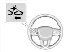
The Collision Alert control is on the steering wheel. Press ⇒ to set the FCA timing to Far, Medium, or Near. The first button press shows the current setting on the DIC. Additional button presses will change this setting. The chosen setting will remain until it is changed and will affect the timing of both the Collision Alert and the Tailgating Alert features. The timing of both alerts will vary based on vehicle speed. The faster the
