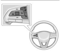
(S): Press to turn the system on or off. The indicator turns white on the instrument cluster when ACC is turned on. **RES+ :** Press briefly to resume the previous set speed or to increase vehicle speed if ACC is already engaged. To increase speed by 1 km/h (1 mph), press RES+ to the first detent. To increase speed to the next 5 km/h (5 mph) mark on the speedometer, press RES+ to the second detent.
