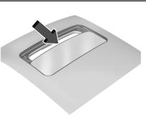
Dirt and debris may collect on the sunroof seal or in the track. This could cause an issue with sunroof operation or noise. It could also plug the water drainage system. Periodically open the sunroof and remove any obstacles or loose debris. Wipe the sunroof seal and roof sealing area using a clean cloth, mild soap, and water. Do not remove grease from the sunroof.
