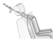
If the position you are using has an adjustable head restraint and you are using a dual tether, raise the head restraint and route the tether under the head restraint and in between the head restraint posts.
