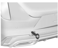
If equipped, carefully open the cover by using the small notch that conceals the rear tow eye socket. Install the tow eye into the socket and turn it until it is fully tightened. When the tow eye is removed, reinstall the cover with the notch in the original position.
