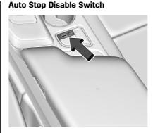
If equipped, the automatic engine Stop/Start feature can be disabled and enabled by pressing A. Auto Stop/ Start is enabled each time you start the vehicle.
