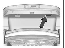
Close the trunk by pulling on the handle. Do not use the handle as a tie-down. Do not press the touch pad while closing the trunk; this will cause the trunk lid to be unlatched.
