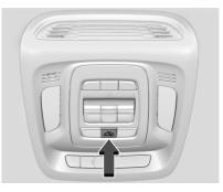
It is recommended that the intrusion and inclination sensor be deactivated if pets are left in the vehicle or the vehicle is being transported. With the vehicle turned off, press in the front overhead console. The indicator light will come on momentarily, indicating that these sensors have been disabled for the next alarm system arming cycle.
