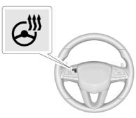
If equipped, press to turn the heated steering wheel on or off. An indicator light next to the button displays when the feature is turned on.
