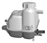
If coolant is visible but the coolant level is not at or above the indicated mark, add a 50/50 mixture of clean drinkable water and DEX-COOL coolant.
