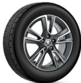
Proxima light-alloy wheel 6J x 16" ET45 for 195/55 R16 tyre
