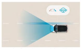
Lane Keeping Assist (LKA): This system uses the front multi-function camera to monitor the lines of the road. In case of an unintended lane departure, it warns you and can apply counter steering torque to guide the car back to the lane.
