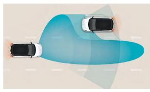
**High Beam Assist (HBA):** Less stress and maximum visibility. HBA not only detects oncoming vehicles but also vehicles in the same lane ahead and switches to low-beam as appropriate.
