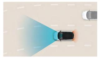
Navigation-based Smart Cruise Control (NSCC): Utilises the state-of-the-art navigation system to anticipate upcoming curves or straights on highways and automatically adjusts speed for safer driving. Also, if activated, the set speed also changes automatically whenever the posted speed limit changes.
