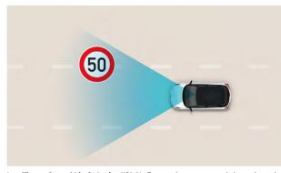
Intelligent Speed Limit Assist (ISLA): External cameras and the onboard navigation system combine to monitor road speed limits, keeping you informed via the navigation screen to keep your pace at a safe speed.
