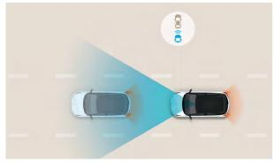
Forward Collision Avoidance (FCA): The front view camera and radar sensors warn drivers of imminent collisions with vehicles and objects, applying the brakes when necessary to avoid collisions. The system includes Junction Assist (Turning) on SE Connect and Junction Assist (Turning/Crossing) on Premium and Ultimate.
