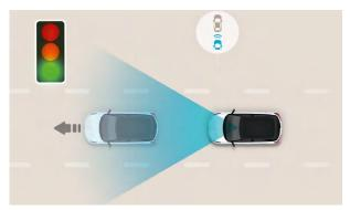
Leading Vehicle Departure Alert (LVDA): This clever feature for city driving alerts the driver when the vehicle in front departs from an idle state, like at a stoplight or in a traffic jam.
