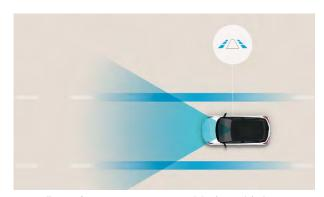
Lane Follow Assist (LFA): Smart sensors and the forward-facing camera detect when the car drifts from the centre of the lane, applying steering torque to maintain road positioning for safety. The car also estimates the trajectory of the vehicle ahead and adjusts its position accordingly.
