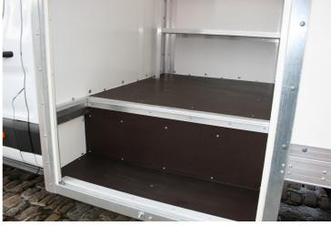
SIDE ROLLER SHUTTER DOOR IS ENTRY TO STORAGE UNIT WITH SHELVING RACKS
