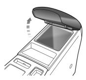
Lift the armrest (as indicated by the arrow) to open the box cover. Put the armrest down to close the centre console armrest box.
