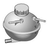
The cooling system should be checked weekly. During the check, the vehicle shall be parked on a flat ground, and the cooling system must be in cold state. If the level is lower than "MIN" mark, open the expansion tank cap of the cooling system and refill the coolant. But the level shall not be higher than "MAX" mark.
