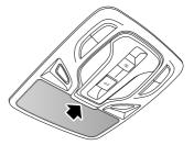
The glasses box is located in the proximity of the front courtesy lamps. Press the panel (as indicated by the arrow) to open the glasses box. Close the glasses box when it is not in use.
