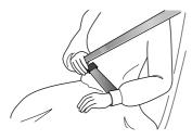
2 Insert the metal tab into the buckle until you hear a "click" sound, which indicates the seat belt is locked tightly.
