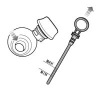
Check the oil level weekly and top up with oil when necessary. Ideally, the oil level should be checked with the engine cold and the car resting on level ground. However, if the engine is running and already getting warm, wait for at least five minutes after switching off the START/STOP switch before checking the level.
