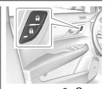
From the inside, press  $\bigcirc$  or  $\bigcirc$ . The indicator light in the switch will illuminate when locked. See *Power Door Locks*  $\Rightarrow$  36.
