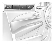
The 1, 2, SET, and (Exit) buttons on the driver door are used to manually save and recall memory settings for the driver seat, outside mirrors, and power tilt and telescoping steering column (if equipped).
