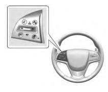
(c): Press to turn the system on or off. A white cruise control indicator comes on.
