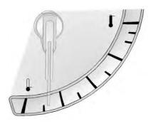
This gauge measures the engine coolant temperature.
