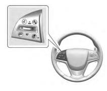
(S): Press to turn the system on and off. A white cruise control indicator appears in the instrument cluster when cruise is turned on.
