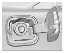
The coupe vehicle has a capless refueling system and does not have a fuel cap. The filling nozzle must be fully inserted and latched prior to starting fuel flow.
