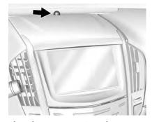
The solar sensor monitors the solar heat.
