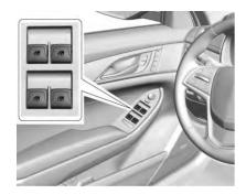
The windows work when the vehicle is in ON/RUN or ACC/ACCESSORY, or when Retained Accessory Power (RAP) is active. See *Retained Accessory Power (RAP)* ⇒ 200.
