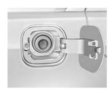
To open the fuel door, push and release the rearward center edge of the door. The fuel door is locked when the vehicle doors are locked. Press on the RKE transmitter to unlock.
