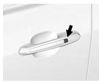
Use the Keyless Access system to lock and unlock the door. When the doors are locked and the Remote Keyless Entry (RKE) transmitter is within 1 m (3 ft) of the driver door handle, press the lock/unlock button. When unlocking from the driver door, the first press unlocks that door; press
