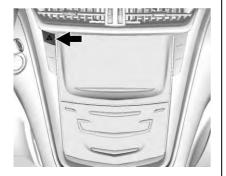
ightharpoole : Press and hold this button for one second to make the front and rear turn signal lamps flash on and off. Release the button for at least one second and press again to turn the flashers off.
