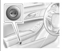
To open the trunk, press on the driver door, press twice quickly on the Remote Keyless Entry (RKE) transmitter, or press the touch pad on the rear of the vehicle after unlocking all doors.
