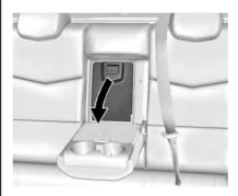
The vehicle has a rear seat pass-through door in the center of the rear seatback. Fold down the center armrest and pull the lever all the way down to release the door.
