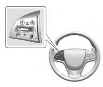
The Collision Alert control is on the steering wheel. Press to set the FCA timing to Far, Medium, Near, or on some vehicles, Off. The first button press shows the current setting on the DIC. Additional button presses will change this setting. The chosen setting will remain until it is changed and will affect the timing of both the Collision Alert and the Tailgating Alert features. The timing of both
