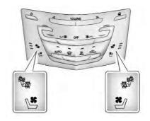
If equipped, the buttons are near the climate controls on the center stack. To operate, the ignition must be in ON/RUN/START.
