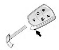
Press the button to remove the key. The key can be used for the driver door, rear folding seats and the rear seat pass-through door.
