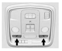
Press or next to each overhead console reading lamp.
