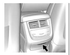
If equipped, press the top of the door to open the storage area on the rear of the center console. If equipped, there is a power outlet inside.
