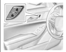
From inside, press of or a. The indicator light in the switch will illuminate when locked. See *Power Door Locks* ⇔ 37.
