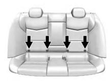
The outboard lower anchors are behind the vertical openings in the seat trim.
