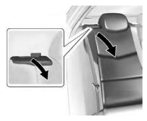
2. Unlock the seatback using the vehicle key in the cylinder.
