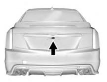
The camera that provides the Rear Camera Mirror (RCM) image is above the license plate, next to the Rear Vision Camera (RVC).
