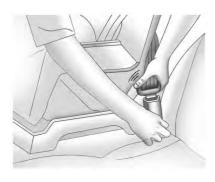
Push the latch plate into the buckle until it clicks. If the latch plate will not go fully into the buckle, check if the correct buckle is being used.
