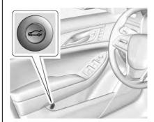
To open the trunk, the vehicle must be off or the shift lever must be in P (Park).
