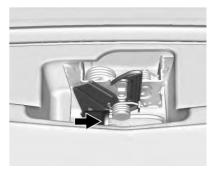
Go to the front of the vehicle to find the secondary hood release handle. The handle is under the front edge of the hood near the center. Push the handle to the right and at the same time raise the hood.
