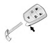
This key, inside the Remote Keyless Entry (RKE) transmitter, is used for the driver door, and rear folding seats and rear seat pass-through door.
