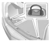
The cargo tie-downs can be used to secure small loads inside the trunk.
