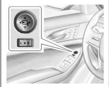
Controls for the outside power mirrors are on the driver door.
