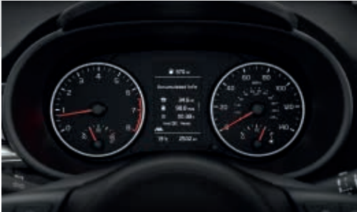
New 4.2 inch colour Supervision digital cluster The vivid colour LCD screen displays a whole range of essential vehicle status and trip data to keep you fully informed.
