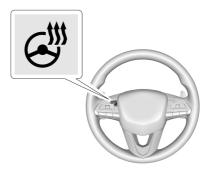
If equipped, press to turn the heated steering wheel on or off. An indicator light next to the button displays when the feature is turned on.
