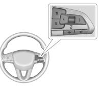
Press  $\leq$  or > to access the cluster applications. Use the thumbwheel to scroll  $\land$  or  $\lor$  through the list of available features. Press the thumbwheel to select. Not all applications will be available on all vehicles.
