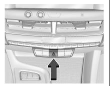
$\triangle$ : Press this button to make the front and rear turn signal lamps flash on and off. Release the button for at least one second and press again to turn the flashers off.
