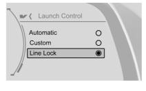
Using the DIC buttons on the right side of the steering wheel, navigate to the Line Lock menu within Launch Control. See Driver Information Center (DIC) (Base Level)
