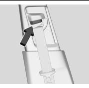
Press the release button and move the height adjuster to the desired position. The adjuster can be moved up by pushing the slide/trim up. After the adjuster is set to the desired position, try to move it down without pressing the release button to make sure it has locked into position.
