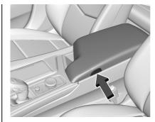
Press the button and lift to access the storage area. There is an accessory power outlet, two USB ports, and an SD card slot inside. See *Power Outlets*  $\Rightarrow$  90 or *USB Port*  $\Rightarrow$  148.
