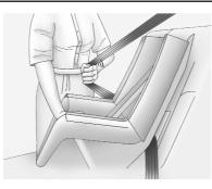
5. Pull the shoulder belt all the way out of the retractor to set the lock. When the retractor lock is set, the belt can be tightened but not pulled out of the retractor.
