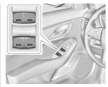
Power windows work when the ignition is on, in ACC/ACCESSORY, or when Retained Accessory Power (RAP) is active. See *Retained Accessory Power* (*RAP*)  $\Rightarrow$  224.
