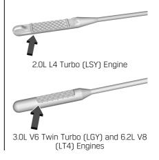
If the oil is below the cross-hatched area at the tip of the dipstick and the engine has been off for at least 15 minutes, add 1 L (1 qt) of the recommended oil and then recheck the level. See "Selecting the Right Engine Oil" later in this section for an explanation of what kind of oil to use. For engine oil crankcase capacity, see *Capacities and Specifications*  $\Rightarrow$  369.
