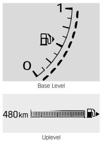
When the ignition is on, the fuel gauge indicates the approximate amount of fuel left in the tank.
