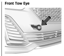
The vehicle is equipped with a tow eye. Only use the tow eye to pull the vehicle onto a flatbed car carrier from a flat road surface. Do not use the tow eye to pull the vehicle from snow, mud, or sand. The tow eye is located under the carpet in the trunk.
