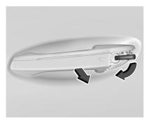
3. Insert the mechanical key in the cylinder.
