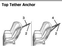
A top tether (3,4) is used to secure the top of the child restraint to the vehicle. A top tether anchor is built into the vehicle. The top tether attachment hook (2) on the child restraint connects to the top tether anchor in the vehicle in order to reduce the forward movement and rotation of the child restraint during driving or in a crash.
