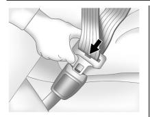
3. Push the latch plate into the buckle until it clicks. Pull up on the latch plate to make sure it is secure.
