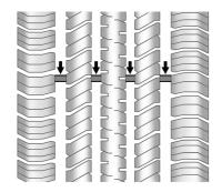
Treadwear indicators are one way to tell when it is time for new tires. Treadwear indicators appear when the tires have only 1.6 mm (1/16 in) or less of tread remaining. See *Tire Inspection*  $\Rightarrow$  *330* and *Tire Rotation*  $\Rightarrow$  *330* for additional information.
