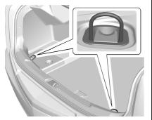
The cargo tie-downs can be used to secure small loads inside the trunk.
