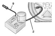
7. Attach the sealant/air hose (2) to the tire valve stem by turning it clockwise until tight.  Plug the power plug (9) into the accessory power outlet in the vehicle. Unplug all items from other accessory power outlets. See *Power Outlets* \$\vdots\$ 90.
