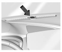
If equipped, the light sensor is on top of the instrument panel or on the windshield near the rearview mirror. Do not cover the sensor, otherwise the headlamps will come on when they are not needed. The system may also turn on the headlamps when driving through a parking garage or tunnel.
