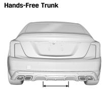
If equipped, the trunk may be opened with a kicking motion under the rear bumper at the location of the projected logo. The remote key must be within 1 m (3 ft).
