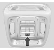
It is recommended that the intrusion and inclination sensor be deactivated if pets are left in the vehicle or the vehicle is being transported. With the vehicle turned off, press in the front overhead console. The indicator light will come on momentarily, indicating that these sensors have been disabled for the next alarm system arming cycle.
