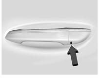
Insert the mechanical key into the slot at the bottom of the handle and push upward all the way until the cover frees. Do not pry or pull on the key.
