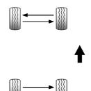
Use this rotation pattern if the vehicle has different size tires on the front and rear.
