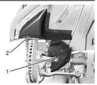
Right Side Front Shown, Left Side Front Similar 1. Front Lower Control Arm Deflector 2. Remove – Front Tire Deflector
