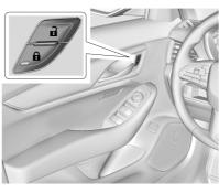
**•** : Press to lock the doors. The indicator light in the switch will illuminate when locked.
