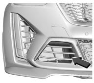
3. Front Brake Cooling Duct
