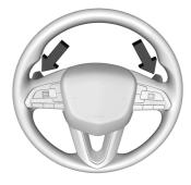
If equipped, vehicles with Tap Shift have controls on the back of the steering wheel to manually shift the automatic transmission.
