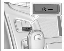
If equipped, the automatic engine Stop/Start feature can be disabled and enabled by pressing  $\triangle$ . Auto Stop/Start is enabled each time you start the vehicle.
