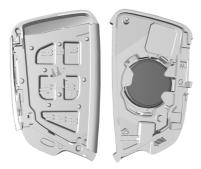
4. Remove the old battery. Do not use a metal object.
