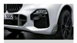
Air Inlet and Front Winglets, Carbon
