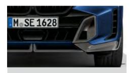
Front Splitter & Air Inlet Trims, Carbon
