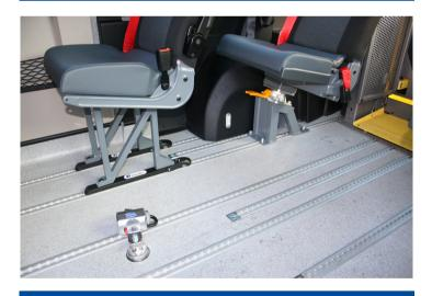
METAL FLOOR TRACKING ALLOWS FOR THE MOVEMENT OF SEATS
