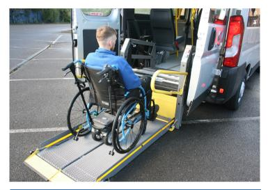
REMOTE CONTROLLED TAIL LIFT ENSURES SAFE ENTRY INTO THE VEHICLE
