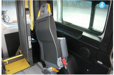
2 REAR SWIVEL CHAIRS CAN BE USED WHEN NO WHEELCHAIR PASSENGER IS TRAVELLING
