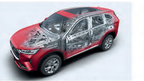
71.61% High-strength Steel Body
