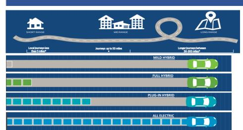
\* Ranges are estimates only and depend on the vehicle, road conditions and driving behaviour.
