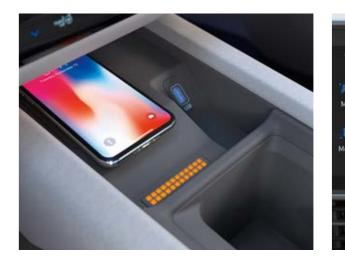
The wireless charger port features Parametric Pixels that signal the charge level of your smartphone at a glance.
