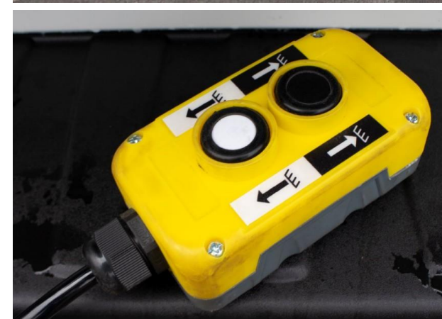
TIPPER IS CONTROLLED VIA YELLOW REMOTE
