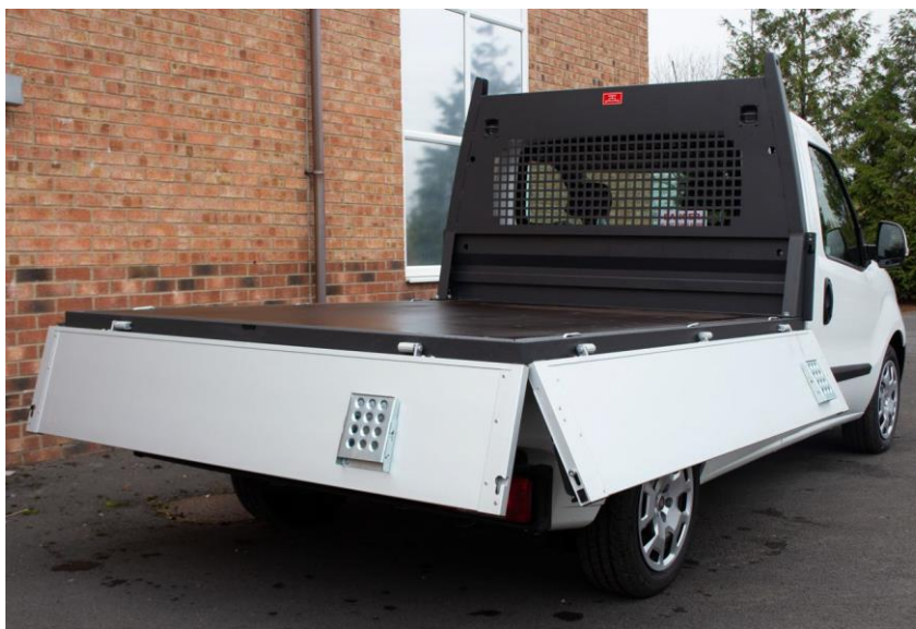
DROP SIDE ALLOWS FOR EASY REMOVAL OF STORED ITEMS
