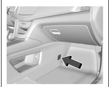
The instrument panel fuse block is in the center console between the driver and passenger seats. To access the fuses, open the fuse panel door, or remove the panel from the passenger side by pulling it out.
