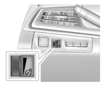
The brightness of the instrument panel lighting and steering wheel controls can be adjusted.
