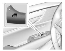
This feature stops the rear passenger window switches from working.
