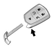
Press the button on the side of the transmitter near the bottom and pull the key out. Never pull the key out without pressing the button.
