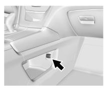
The vehicle has two accessory power outlets: one on the lower center floor console and one in the rear cargo area.
