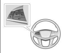
(c): Press to turn the system on and off. A white indicator appears in the instrument cluster when cruise is turned on
