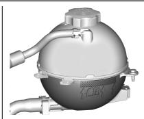
Check to see if coolant is visible in the coolant surge tank. If the coolant inside the coolant surge tank is boiling, do not do anything else until it cools down. If coolant is visible but the coolant level mark is not at or above the indicated mark, add a 50/50 mixture of clean, drinkable water and DEX-COOL coolant. Be sure the cooling system is cool before this is done. See *Engine Overheating*  $\Rightarrow$  261.
