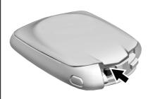
Separate the two halves of the transmitter using a flat tool inserted into the bottom center of the transmitter. Do not use the key slot.
