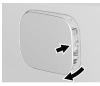
To open the fuel door, push and release the rearward center edge of the door.
