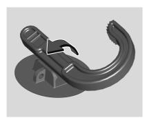
1. Insert one side of the load floor hook into the holder.
