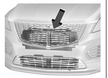
The vehicle may have a shutter system designed to help increase fuel economy. Keep the shutter system clean for proper operation.
