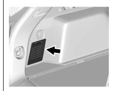
The rear compartment fuse block is in the cargo area, on the driver side of the vehicle behind the lower trim panel. To open, turn the latch with a flat-bladed tool and pull the trim panel from the edges to fold it down.
