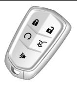
**a**: Press to lock all doors and the fuel door. The turn signal indicators may flash and/or the horn may sound on the second press to indicate locking. See *Vehicle Personalization*
