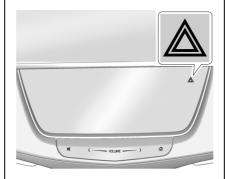
≜: Touch ≜ on the center stack to make the front and rear turn signal lamps flash on and off. Touch again to turn the flashers off.
