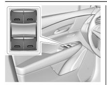
The power windows work when the ignition is on, in ACC/ACCESSORY, or when Retained Accessory Power (RAP) is active. See *Retained Accessory Power (RAP)* ⇒ 176.
