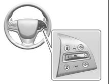
$\wedge$  or  $\vee$ : Press the five-way control to move up or down in a list.
