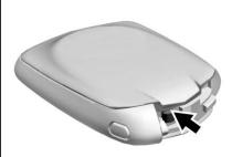
2. Separate the two halves of the transmitter using a flat tool inserted into the bottom center of the transmitter. Do not use the key slot.
