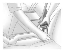
Push the latch plate into the buckle until it clicks. If the latch plate will not go fully into the buckle, check if the correct buckle is being used.
