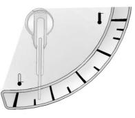
This gauge measures the engine coolant temperature.
