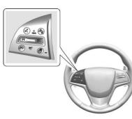
(5): Press to turn the system on and off. A white cruise control indicator appears in the instrument cluster when cruise is turned on.
