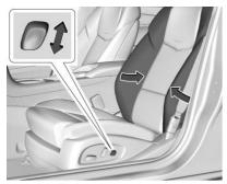
If equipped, to increase or decrease the back bolster support, press and hold the lumbar control up and down.
