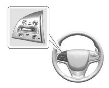
(5): Press to turn the system on or off. The indicator turns white on the instrument cluster when ACC is turned on. **+RES :** Press the control up briefly to resume the previous set speed or to increase vehicle speed if ACC is already engaged. To increase speed by 1 km/h (1 mph), press +RES up to the first detent. To increase speed to the next 5 km/h (5 mph) mark on the speedometer, press +RES up to the second detent.
