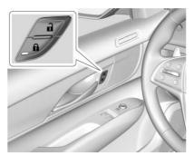
From the inside, press **r** or **a**. The indicator light in the switch will illuminate when locked. See *Power Door Locks*  $\Leftrightarrow$  36.
