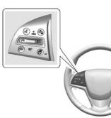
(5): Press to turn the system on and off. A white cruise control indicator appears in the instrument cluster when cruise is turned on.
