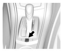
The automatic engine stop/start function can be disabled and enabled by pressing the switch with the (A)
