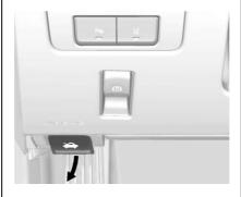
1. Pull the hood release handle inside the vehicle. It is on the lower left side of the instrument panel.
