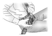
If the webbing locks in the latch plate before it reaches the buckle, tilt the latch plate flat to unlock.
