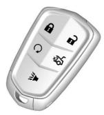
**⊋** : Press to lock all doors and the fuel door. The turn signal indicators may flash and/or the horn may sound to indicate locking on the second press. See *Vehicle Personalization* ⇔ 136.
