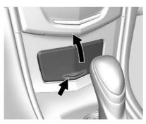
To access, press on the cover and release. There is an accessory power outlet inside. See *Power Outlets*  $\Rightarrow$  *109*.
