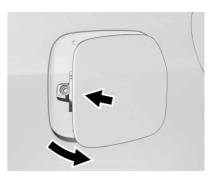
The fuel door is locked when the vehicle doors are locked. Press an on the RKE transmitter to unlock.
